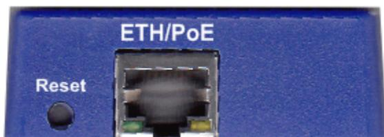
There are specific commands you can send to the unit by holding the Reset button for a specified amount of time.
